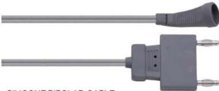
SILICONE BIPOLAR CABLE SB-710-170-3M SB-710-175-5M Instrument Connector : USA 2-Pin Plug Generator Connector : Pin Distance 29mm Compatibility: Valleylab, EMO, Doly
